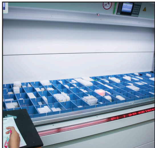
Vertical, barcode controlled inventory storage
