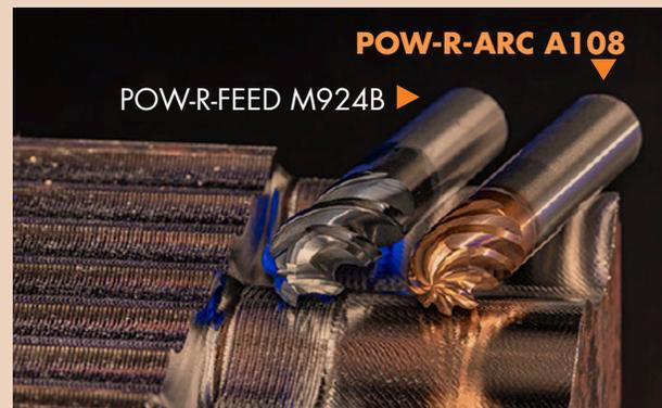
The tools: The POW-R-FEED M924B (left, 3/4 in. dia., 4-flute ball end, 1 in. LOC) v. the POW-R-ARC A108 (right, 3/4 in. dia., 8-flute ball end, 1 in. LOC) Material: A2 at 60 HRc. Using the same stepover value, the new POW-R-ARC 8-flute tool provides a superior 3D contour cut 5x faster, with barely visible ridges (far right) and very little finish work.
